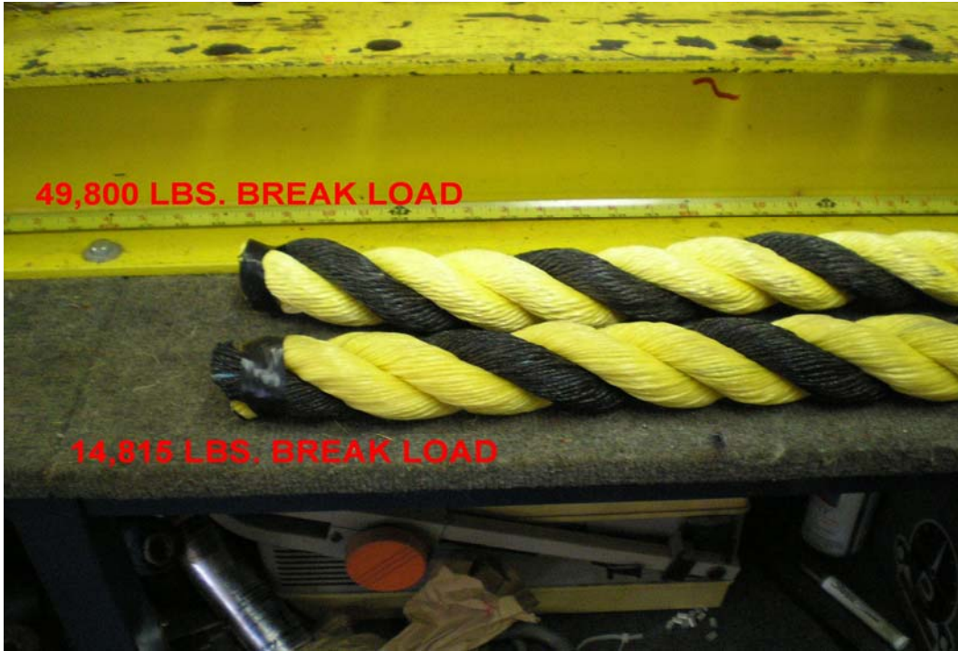
Fig. 3 Top. normal 2 inch dia. polypropylene rope, minimum break strength 49,800 lbs. Bottom, deceptive "polypropylene" rope, actual break strength 14,815 lbs.
