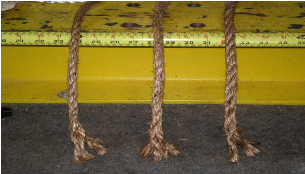
Fig. 6 Three Undersize or Understrength 1/2 inch Diameter Manila Rope
