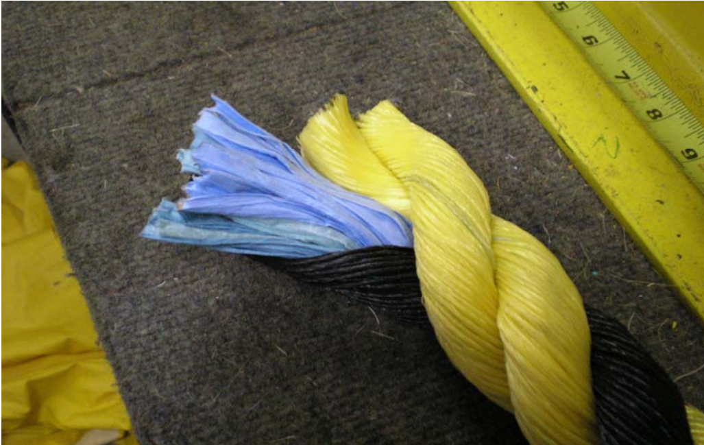
Fig. 1 Photo of deceptive “polypropylene” rope, showing blue non-woven cloth filler in interior of strand.
