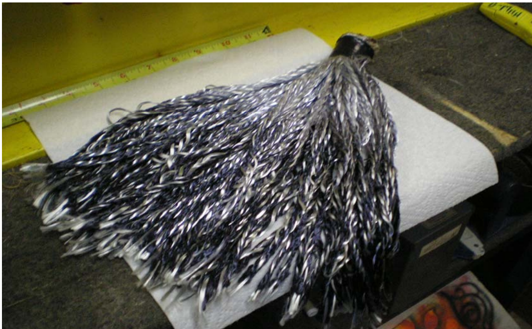
Fig. 4 Deceptive "nylon" strand after the dye test. The black strands are nylon, but the white strands are polyester
